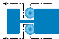
Adjustable draw bar limit for side brushes
